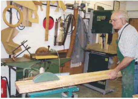
▲ Pic.1 Mike ripped down a 225mm-wide board to make two 100 x 50mm sections for the stiles
